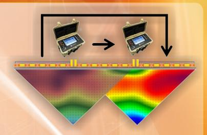
Standard multi-electrode cable set supplied with SibER-64 (5m spacing) allows profile length up to 315m. Profiles could be continued indefinitely by moving the first cable segment of the first layout to the last place in the next layout. Optionally, cable sets with smaller or larger electrode spacing are offered (1, 2, 10, 15, and 20m).
