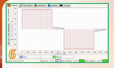
• Measuring sequence can contain up to 8 arrays of different configuration. User can choose the composite pattern and run one cycle of all the measurements, and then process the data as if the measurements were made with several different patterns. [7]
