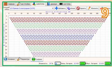
• During data collection apparent electrical resistivity (ER) and induced polarization (IP) data are interactively shown on display as color profile image, profile layers or sounding curves. [10, 11]
