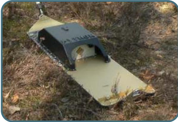
**Python-3** is a portable digital wireless ground penetrating radar carried by a single operator, especially used for deep survey (up to 50 meters in favorable ground). Georadar consists of central segment (100 MHz operating frequency) and 4 additional antenna plates to change operating frequency to 50/38/25 MHz
