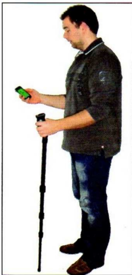
The entire Rover UC package consists of a sensor configured like a standard hiking stick and an Android-based cell phone.
